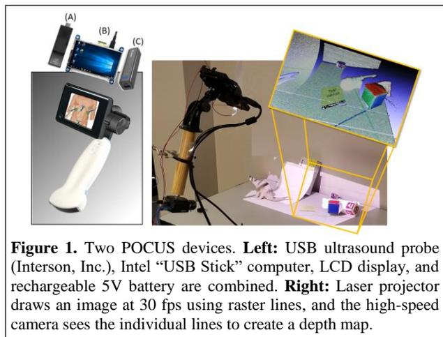
**Figure 1.** Two POCUS devices. **Left:** USB ultrasound probe (Interson, Inc.), Intel “USB Stick” computer, LCD display, and rechargeable 5V battery are combined. **Right:** Laser projector draws an image at 30 fps using raster lines, and the high-speed camera sees the individual lines to create a depth map.
